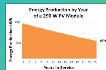
These models of irradiance and temperature are applied to the seven key module characteristics, and the impact on each one is combined without weighting to obtain the 25 year LEP. Degradation over time is based on warranty terms, not accelerated testing. We normalize the energy value using the total irradiation accumulated per square meter in 25 years. In this way, PV modules can be compared as if installed side-by-side irrespective of orientation, tracking configuration or inverter choice.
